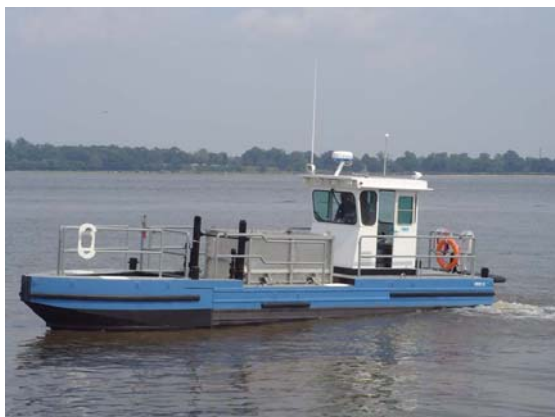
Figure 10: Floatables Skimming Vessel
